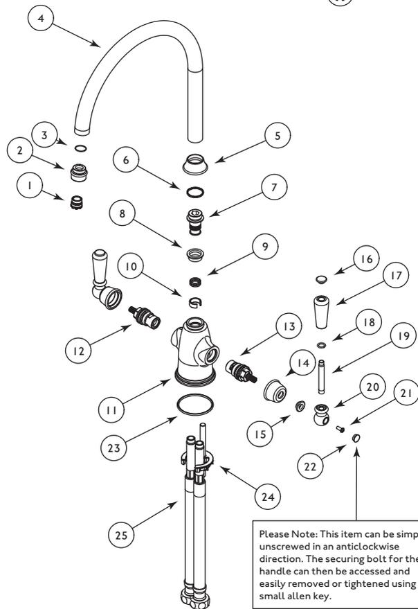
Please Note: This item can be simply unscrewed in an anticlockwise direction. The securing bolt for the handle can then be accessed and easily removed or tightened using a small allen key.
