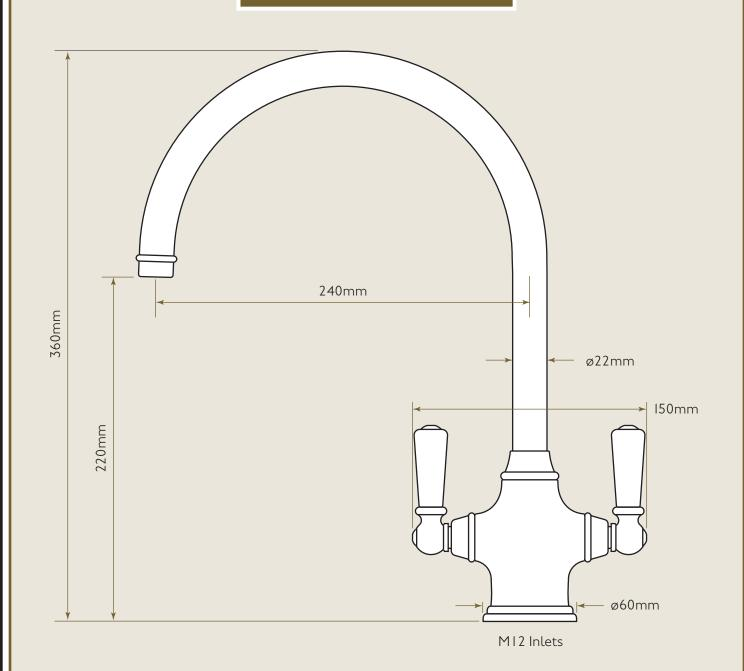
RECOMMENDED HOLE SIZE 35mm Supplied with 400mm flexi tails ( $G^{3}$ /4" connection)
