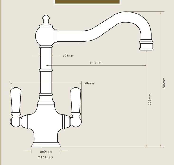
RECOMMENDED HOLE SIZE 35mm Supplied with 400mm flexi tails (G  $^{3}\!4$ " connection)
