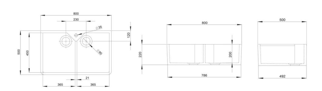
NB. Due to manufacturing processes this sink may have a dimension tolerance as follows
