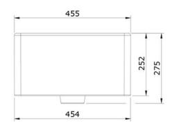
NB: Due to manufacturing processes this sink may have a +/- 5mm tolerance on overall measurements, further variances can also occur dependent on specific areas of the sink.
